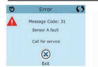
Sensor A Fault, Sensor B Fault - Sensor A: M031\*\*, Sensor B: M032\*\*
