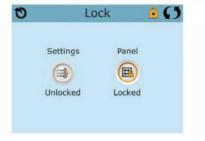
The control can be restricted to prevent unwanted use or temperature adjustments.
