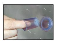
**Step 6.** Slide the plastic filter back in the Jet.
