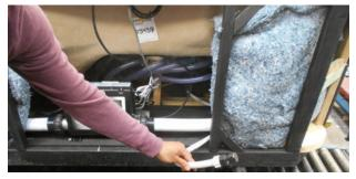
Reattach and screw panels back in. (Front door is installed first, then install the corner panels.)
