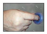
Step 5. Tap the filter and/or blow out the debris to ensure all holes are clear.
