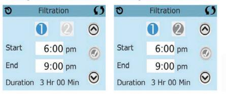
Press "1" to view Filter 1. Press "2" once to view Filter 2. Press "2" again to turn Filter 2 ON or OFF.
