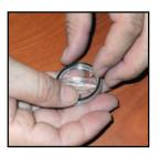
**Step 9.** Insert the plastic spout into the jet body.
