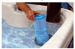
Unscrew the cartridge and remove it.
